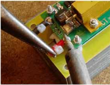
Step 4 Remove lead ends.
