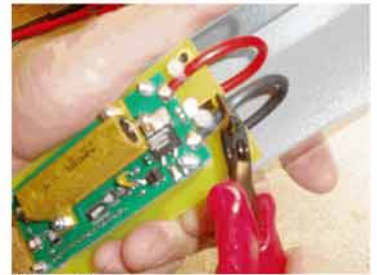
Step 3 Cut and remove old leads.
