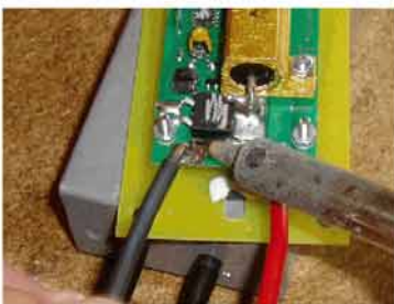
Step 10 Solder into position (WARNING: Observe polarity).
