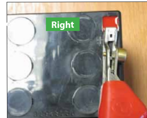
Grip clips tightly around tab terminals
