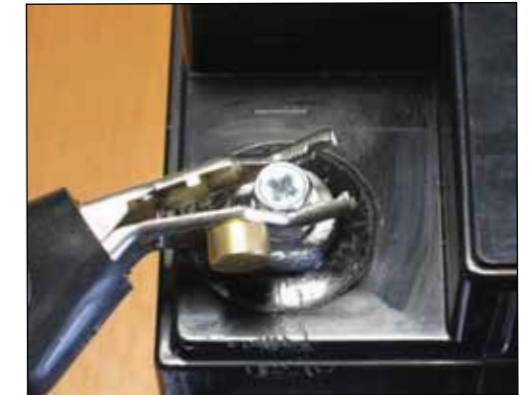
Do not connect clips to high resistance bolts
