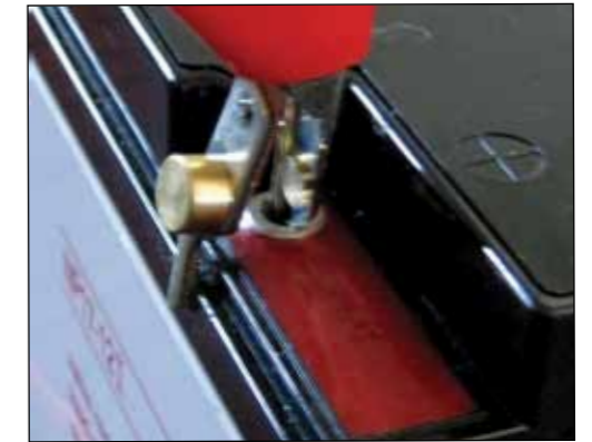
Push clips tightly inside battery terminals
